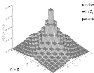
random vector  $Z = (Z_1, Z_2, ... Z_n)$ with  $Z_i = G_{1,i} - G_{2,i}$  (stoch. indep.); parameter q for all G<sub>1i</sub>, G<sub>2i</sub> equal
