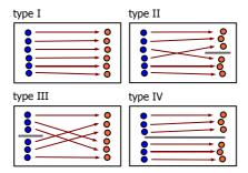
**Fig. 1.** Different Pareto set and Pareto front type combinations: One Pareto set and one Pareto front (type I), one Pareto set and multiple Pareto front parts (type II), multiple Pareto subsets and one Pareto front (type III), and multiple Pareto subsets and Pareto front parts (type IV). Type III problems are rarely investigated, although they potentially provide multiple preimages for every objective vector of interest.
