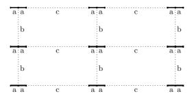
**Fig. 2.** Blue print of the initial test problem: Each subset of the Pareto set is a line of length 2a. Parameter b specifies the vertical distance between neighboring Pareto subsets, whereas parameter c specifies the distance to the next Pareto subset on the horizontal line. Each Pareto subset maps to the same Pareto front.
